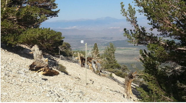
Figure 8. Placement of temperature and snow sensors within forest populations of interest allows researchers to evaluate the effectiveness of regional or gridded models for their sites.
