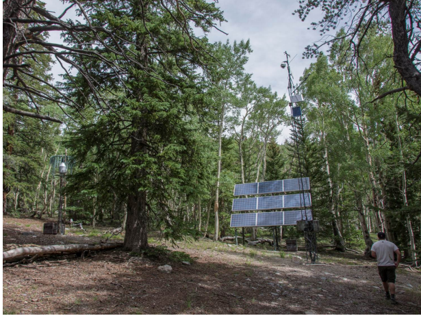
Figure 10. This remote station in Nevada's Snake Range is monitoring climate variables such as precipitation, temperature, radiation, and humidity, as well as tree sap velocity for three species and soil moisture/temperature. General forest conditions are also qualitatively assessed using hourly imagery.
