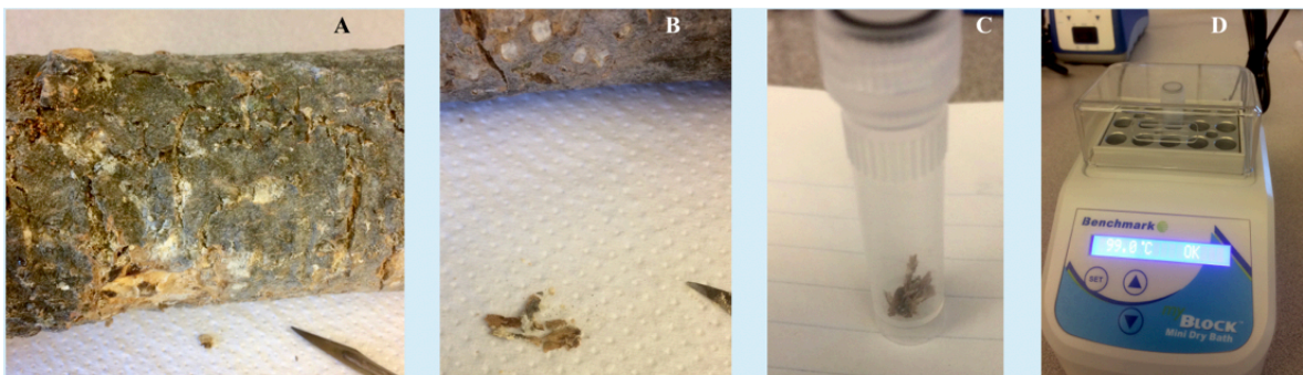
Figure 1: A: example of branch sample from where small pieces of wood were taken for DNA extraction (B,C). D: Incubation of tube with wood samples in chelex 100 5% in portable heat block.
