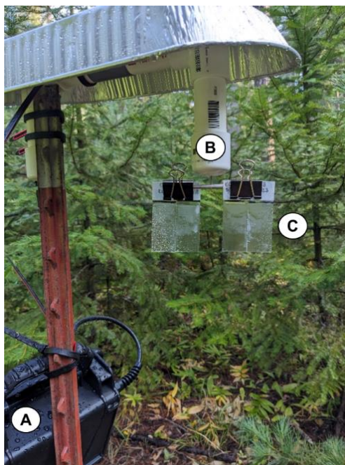
Figure 2: Mechanical spore trap (based on a design by Dr. Walt Mahaffee, Oregon State University). A) 12-Volt battery enclosed in a waterproof plastic case. B) Battery-powered spinning motor attached to an aluminum sampling arm. C) Rotating arm holding four glass slides coated with petroleum jelly that are attached using binder clips.
