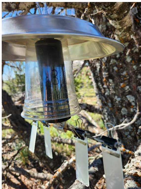
Figure 1: Motorized spore trap used to capture aerial inoculum of Cronartium ribicola , the causal agent of white pine blister rust disease on five-needle white pine trees.
